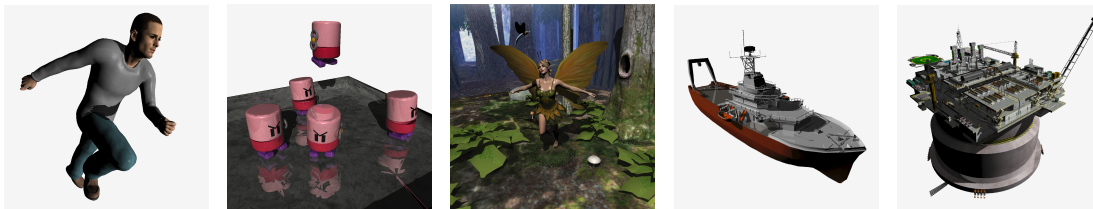
Figure 1: Dynamic and CAD models entirely ray-traced on the GPU with our novel grid construction algorithm. From left to right: running character Ben (78K triangles, 13.3fps with shadows), animated wind-up toys (11k triangles, 28.9fps with shadows and 7.8fps with reflections), fairy dancing in a Forest scene (174k triangles, 2.8fps with shadows), static Boat model (50K triangles, 11.7fps with shadows and 4.1fps with reflections) and static MonoBR oil platform (112K triangles, 5.6fps with shadows and 1.4fps with reflections)
