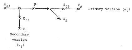
In this example there is one secondary version with two active instances and five active instances of the primary version.  $R_{01}$ ,  $R_{02}$  and  $R_{11}$  are read-only versions, and  $C_0$  and  $C_1$  are the current instances of the two versions.  $\mathcal D$  represents the most recent disc instance (created by a call of flush) and  $A_0$  represents a currently active alternative instance created by a call of indivis that has not yet completed.
