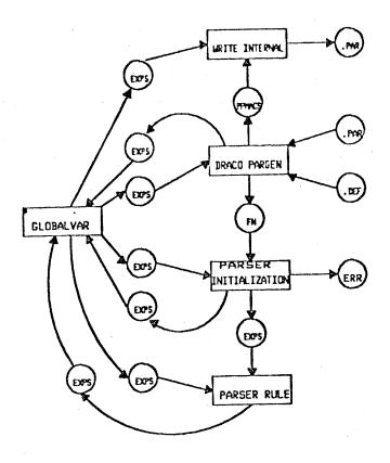
Figure 3: JSD PARGEN System Specification Diagram
